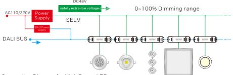
1. Connection Diagram for High Power LED:
