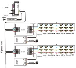
3. Repeaters connected to LED Dimmer as follows:
