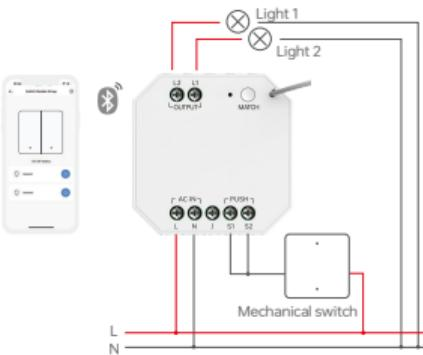
3. Two push switches control one relay each.
