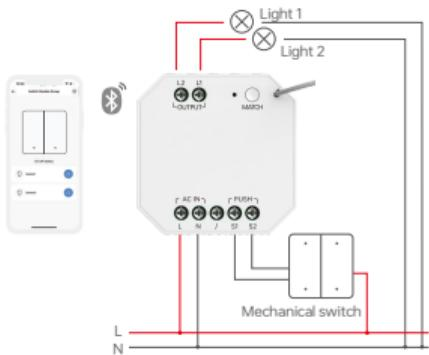
2. One mechanical switch controls two relays.
