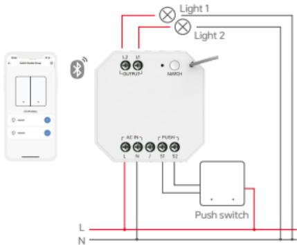
4. One push switch controls two relays.
