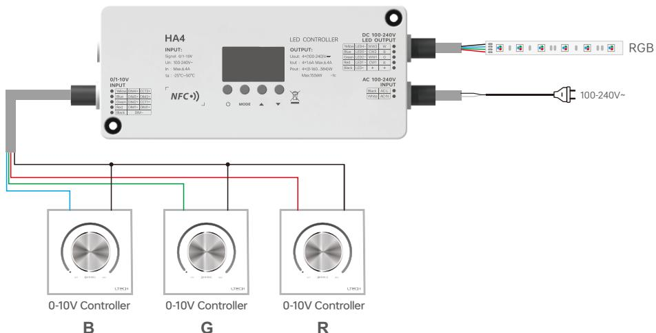
6. Connect one RGBW light, with four controllers separately controlling the R, G, B, and W channels.
