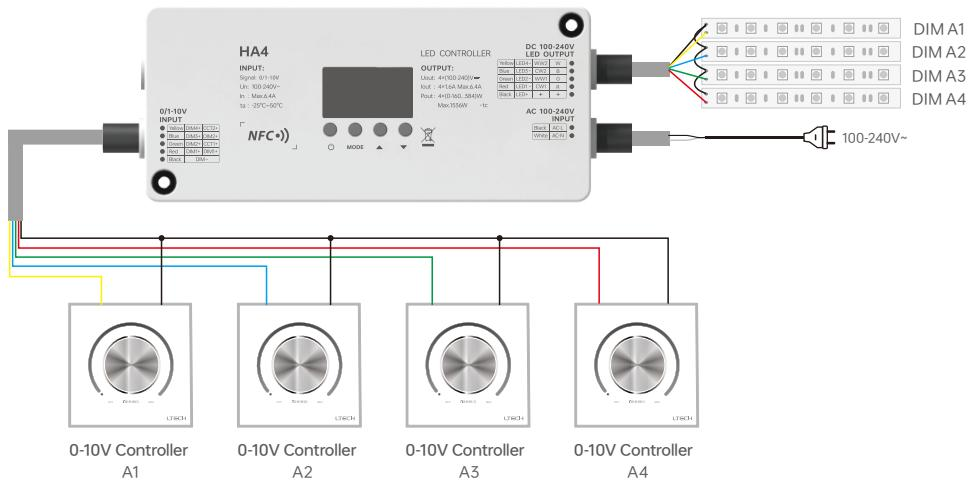
2. Connect four dimmable lights simultaneously, with one dimmer controlling all four lights at once.
